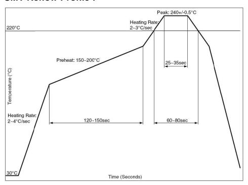
The reflow profile shown above should not be exceeded, since excessive temperatures or transport times during reflow can damage the module. Cooling temperature fall rate: max  $3^{\circ}$ C / sec
